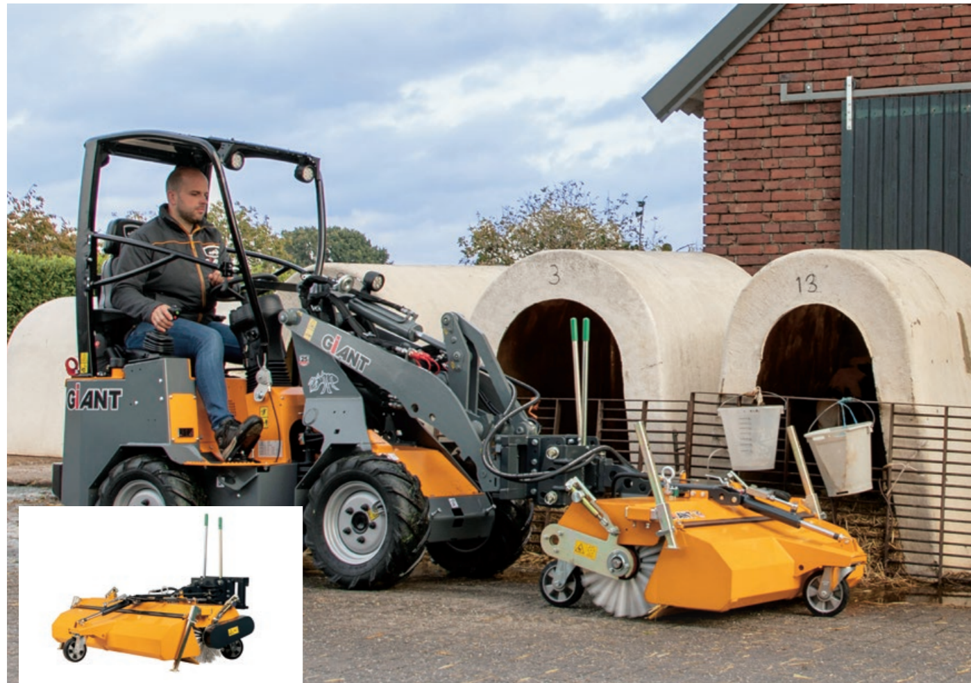
SWEeper Simplex Width: 120 cm Options: hydraulic emptying, hydraulic angling, side brush
