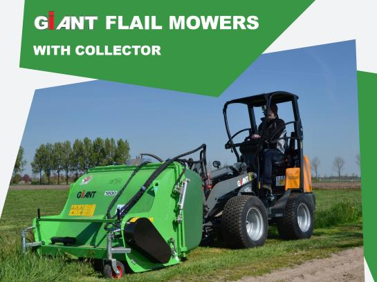
Suitable for mowing, verticutting and removing grass rests, leaves, branches and manure in order to have your lawn or pasture perfectly cleaned and refreshed. Also excellent suitable for public works and sports complexes. The gearbox is supplied with overrun clutch for users and machine safety.
